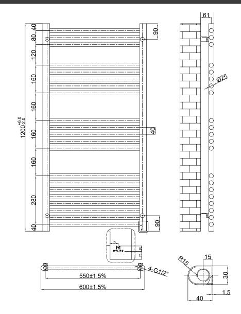
Please note due to manufacturing tolerances pipe centres may vary by +/- 10mm, we recommend that pipe work is not altered until your towel rail / radiator is on site. The information contained on this page was correct at date of issue. Fitting dimensions are provided as a guide only. We pursue a policy of continuing improvement in design and performance of our products and so reserve the right to change specifications without prior notice.
