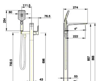
Brass Body CuZn40Pb2, EN CW617N (equivalent to BS CZ122) Construction
