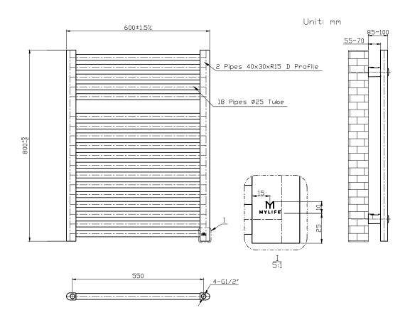
Please note due to manufacturing tolerances pipe centres may vary by +/- 10mm, we recommend that pipe work is not altered until your towel rail / radiator is on site. The information contained on this page was correct at date of issue. Fitting dimensions are provided as a guide only. We pursue a policy of continuing improvement in design and performance of our products and so reserve the right to change specifications without prior notice.
