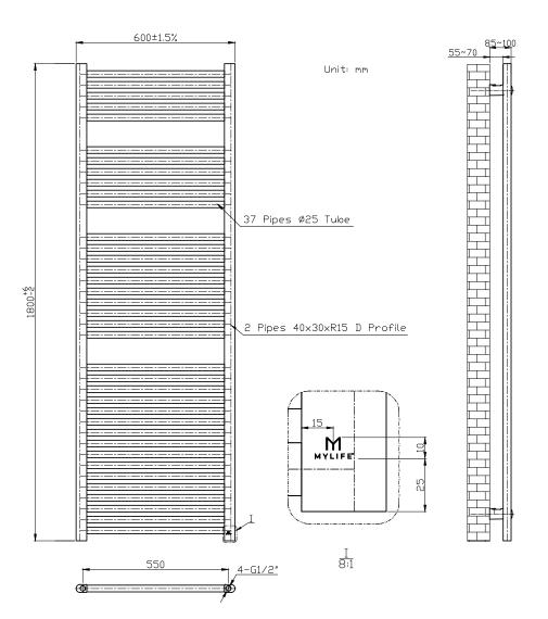
Please note due to manufacturing tolerances pipe centres may vary by +/- 10mm, we recommend that pipe work is not altered until your towel rail / radiator is on site. The information contained on this page was correct at date of issue. Fitting dimensions are provided as a guide only. We pursue a policy of continuing improvement in design and performance of our products and so reserve the right to change specifications without prior notice.
