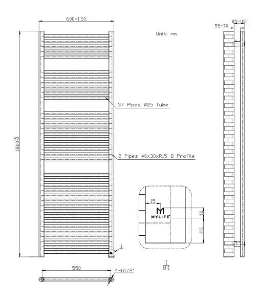
Please note due to manufacturing tolerances pipe centres may vary by +/- 10mm, we recommend that pipe work is not altered until your towel rail / radiator is on site. The information contained on this page was correct at date of issue. Fitting dimensions are provided as a guide only. We pursue a policy of continuing improvement in design and performance of our products and so reserve the right to change specifications without prior notice.
