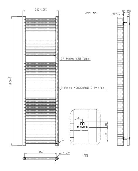
Please note due to manufacturing tolerances pipe centres may vary by +/- 10mm, we recommend that pipe work is not altered until your towel rail / radiator is on site. The information contained on this page was correct at date of issue. Fitting dimensions are provided as a guide only. We pursue a policy of continuing improvement in design and performance of our products and so reserve the right to change specifications without prior notice.
