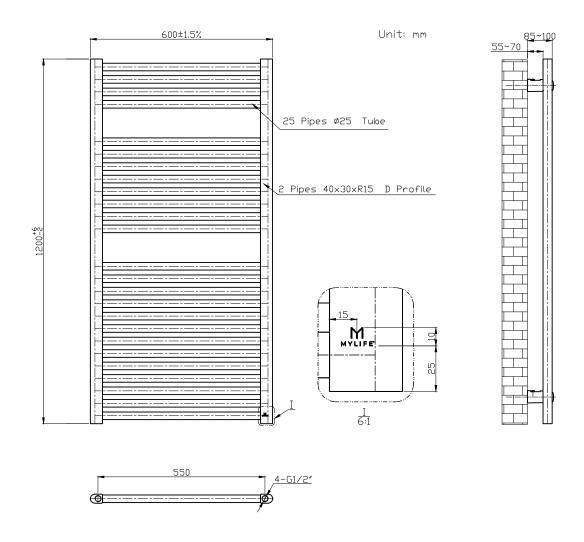
Please note due to manufacturing tolerances pipe centres may vary by +/- 10mm, we recommend that pipe work is not altered until your towel rail / radiator is on site. The information contained on this page was correct at date of issue. Fitting dimensions are provided as a guide only. We pursue a policy of continuing improvement in design and performance of our products and so reserve the right to change specifications without prior notice.
