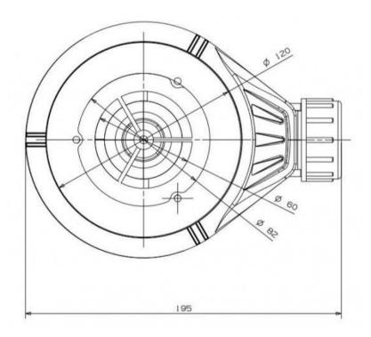
Flow Rate: With 15mm Water: 42L / min Temp. Max: 100°c
