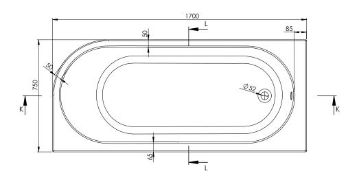
Birr 1700 x 750mm Left Hand Bath Size: L 1700 x W 750 x H 400mm Can Be Drilled For Tap Holes
