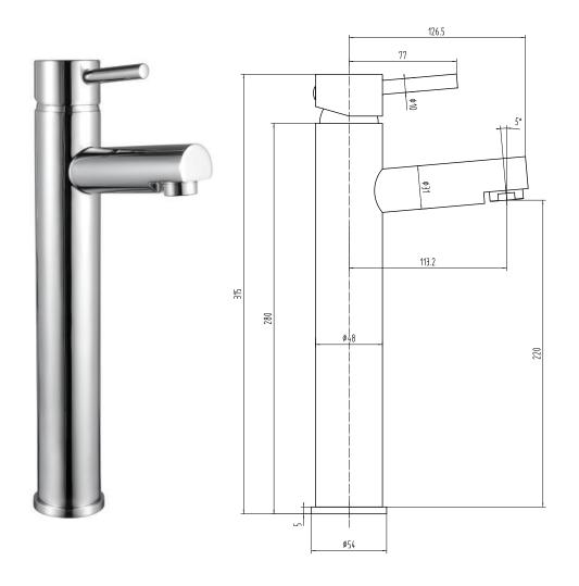
Construction Brass Body CuZn40Pb2, EN CW617N (equivalent to BS CZ122)
