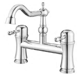
Finishes Product Type Water Pressure Plumbing Systems Standards Cartridge Fitting Guarantee Brass Body (CuZn40Pb18) Zinc alloy Handle Chrome plated to BS EN 248 Traditional Min. 0.5 bar, Max. 6.0 bar Suitable for all plumbing systems Complies with BS5412, BS EN200 Compression Cartridge 3/4" BSP 10 years against manufacturing faults (3 Years on Serviceable Parts).
