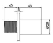
ConstructionBrass Body (CuZn40Pb18)FinishesChrome plated to BS EN 248
