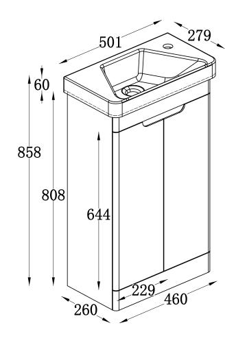
SIZE: H 858 x W 500 x D 280mm TAP HOLE(S): One BASIN MATERIAL: Ceramic UNIT FINISH: Gloss/Matt (No Overflow, Needs Unslotted Waste)
